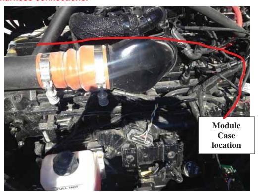
**4)** On the Ag Diesel Solutions harness, the female injector connector located closest to the Ag Diesel Solutions module case will connect to the male injector connector wiring located closest to the flywheel-side of the engine.
