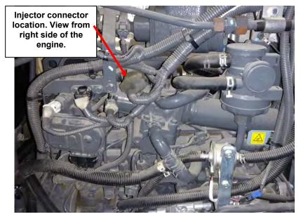
**2)** Unplug the stock injector connector. Press and hold the release tab on the connector and gently pull the connector apart.
