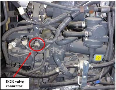
6) Unplug the stock EGR valve connector. Press and hold the release tab on the connector and gently pull the connector apart.
