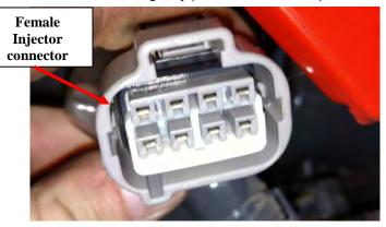
**3)** On the Ag Diesel Solutions module harness, the grey 8 pin male injector connector will connect to the female injector connector fixed on the engine. The Ag Diesel Solutions module harness can be routed along existing wire loom.
