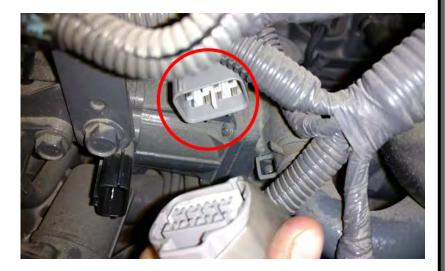
**4)** On the module harness, the 8 pin female Injector connector will now connect to the factory male Injector connector that was unplugged from the engine in step 3.
