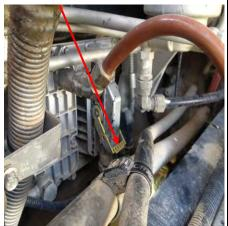
3) Connect the male plug from the new module harness into the ECM.
