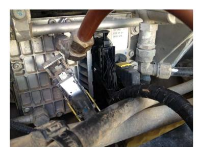
4) Connect the new female harness into the stock male plug located on the engine harness. Squeeze the connector together and then press the Locking Lever to Latch the connector together.
