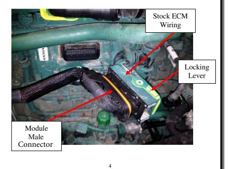
**4)** Plug the module female harness connector into the stock male connector located on the ECM. Press the connector together and then rotate the locking lever to latch the connector to the ECM.
