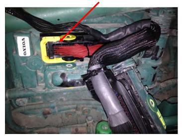
Route the power and ground wires to the alternator. The red wire should connect to a +12 volt constant source. The black wire should connect to a good, clean ground.
