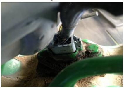
**3)** Plug the male injector connector from the Ag Diesel Solutions module harness into the stock female connector on the engine.
