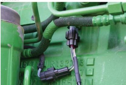
**6)** Plug the male fuel rail sensor connector removed in step 5 to the male connector on the Ag Diesel Solutions module harness. Plug the male fuel rail sensor connector from the Ag Diesel Solutions module harness into the stock fuel rail sensor located on the common fuel rail.
