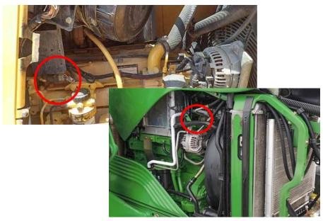
**2)** Unplug the stock injector connector from the engine head. Squeeze the release tabs on each side together to remove the connector.
