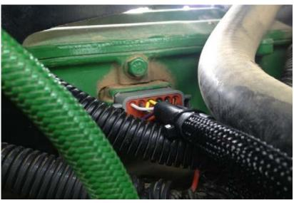
**4)** Plug the factory male injector connector from the engine harness that was removed in Step 2, to the female injector connector from the Ag Diesel Solutions module harness.
