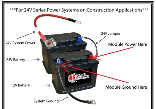
Module power and ground must be hooked to the 12V side of a 24V series power system for the module to function properly. Module ground lead needs to be hooked to the system ground which will be the battery with its ground strap connected to the frame of the machine NOT the jumper running between batteries. The module power lead needs to be hooked up to the positive terminal WITH the jumper (on same battery), NOT the 24V System power terminal. Please see illustration above.
