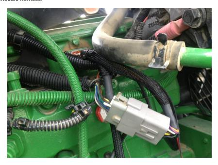
**5)** Locate the fuel rail sensor and unplug it. It is connected to the bottom side of the common fuel rail on the opposite side of the engine as the injector connector.
