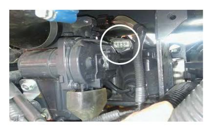
**2)** Unplug the stock injector connector. Press and hold the release tab on the connector and gently pull the connector apart.
