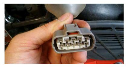
**3)** On the Ag Diesel Solutions module harness, the 10 pin male injector connector will plug into the female injector connector fixed on the valve cover. The Ag Diesel Solutions module harness can be routed along existing wire loom.
