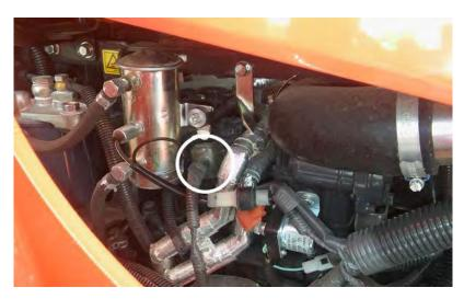
**6)** Unplug the stock EGR valve connector. Press and hold the release tab on the connector and gently pull the connector apart.
