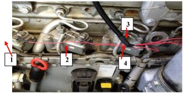
8) Continue routing the wiring toward the transmission-side of the engine.
