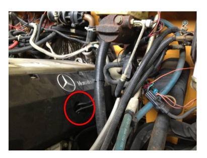
5) Route the module harness wiring in order from 1-8, as shown below. The #1 tag will start at the Unit Injector closest to the engine fan.
