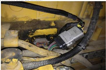
**4)** Locate the MAP Sensor on the top of the passenger side of the engine. Unplug the stock MAP Sensor and plug the male connector into the stock female connector. Plug the stock male connector into the female connector of the module.
