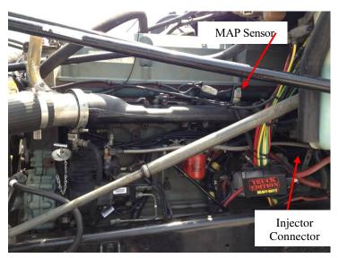
2) Unplug the stock injector connector. Push the red locking tab on the connector to one side. Press the black harness release lever and pull the injector harness apart.
