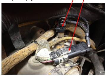
7) Route Switch through firewall and plug into module as shown
