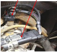
**4)** Locate the MAP sensor on the intake manifold on the driver's side of the engine. Refer to the diagram on Page 2 for approximate location.
