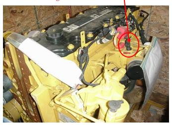
5) Disconnect the MAP Sensor and plug the male from the module into the stock MAP/Boost Sensor.
