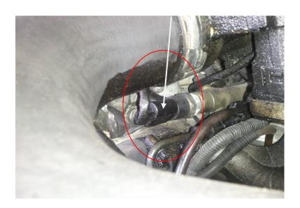
3) Plug the male side of module harness into the factory female plug, next plug female side of harness into fuel pressure sensor.
