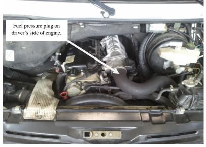
2) Unplug the fuel pressure sensor plug located at the end of common rail on driver's side of engine as shown in the picture.
