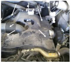
4) Once cover is removed locate Fuel pressure relief valve on back of engine on passenger side.
