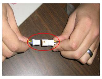
6) Remove the bypass plug from the Ag Diesel Solutions harness, and plug the harness into the module.
