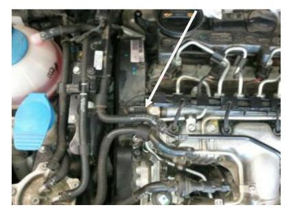
3) Unplug Fuel pressure sensor plug and plug module harness into sensor, next plug factory sensor plug into module harness.
