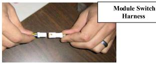
**9)** Remove the bypass plug from the Ag Diesel Solutions harness, and plug the harness into the module.
