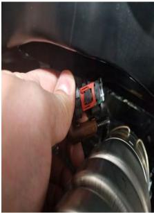
**4)** Connect the male plug from the module into the stock female fuel pressure sensor.
