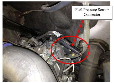
Plug the Female Connector from the module into the Stock Duramax male connector. Plug the Stock Duramax female connector to the male connector from the module. The fuel pressure plugs are located closest to the module case on the new harness.
