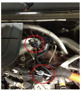
5) Route the Switch through firewall and plug into module as shown below
