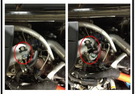
Plug the male MAP Sensor connector from the module harness into the Stock MAP Sensor. Plug the female MAP Sensor connector into the Stock MAP Sensor male connector. Note: The MAP Sensor plugs are located at the end of the harness, furthest away from the module case.
