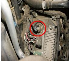
2) Disconnect the Fuel Pressure Sensor.
