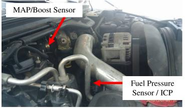
1) Locate Fuel Pressure sensor on the passengers side of the engine as shown in pictures above and below.
