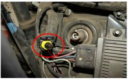
3) Check inside the Fuel Pressure Sensor for a plastic insert. If there is a plastic insert, you will need to remove it and place it over the stock Fuel Pressure Sensor plug as shown below.
