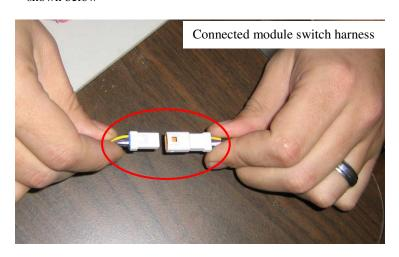
10)) Remove the bypass plug from the Ag Diesel Solutions harness, and plug the harness into the module.
