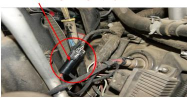
6) Locate the Map sensor on the passenger side of the engine and disconnect it. It is located next to the engine oil fill cap.
