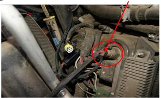
**5**) Connect the Stock Ford connector to the Male Connector from the module.
