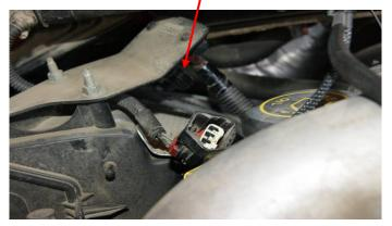
7) Connect the Female plug from the module into the sensor.
