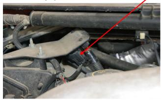
**8)** Connect the Stock MAP sensor connector into the Male Map sensor plug on the module harness.
