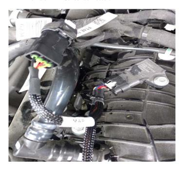
**5)** Disconnect the Factory Female T-MAP Sensor connector from the T-MAP Sensor.
