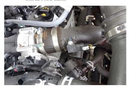
**6)** Utilize the portion of the ADS harness labeled T-MAP. Connect the ADS Female connector to the T-MAP Sensor. Then connect the ADS Male connector to the Factory Female T-MAP Sensor connector.
