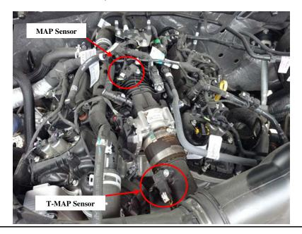
**3)** Disconnect the Factory Female MAP Sensor connector from the MAP Sensor.
