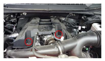
2) With the cover removed, locate the MAP & T-MAP Sensors. The MAP Sensor can be found on top of the intake manifold. The T-MAP Sensor can be found near the throttle body inlet.
