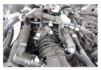
**4)** Utilize the portion of the ADS harness labeled MAP. Connect the ADS Female connector to the MAP Sensor. Then connect the ADS Male connector to the Factory Female MAP Sensor connector.
