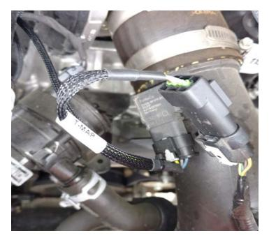
7) Remove the bypass plug from the Ag Diesel Solutions harness, and plug the harness into the module.
