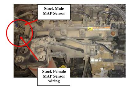
**8)** Connect the new female MAP sensor connector into the stock male MAP sensor. Connect the new male MAP sensor connector into the stock Female MAP sensor wiring.
