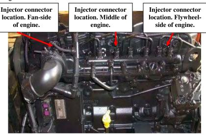
**2)** Disconnect all 3 sets of stock injector connectors. Press the release tab on the connector and gently pull the connector apart.
