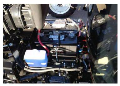
**10)** Plug the Harness into the module. Mount the module with supplied zip ties away from any excessive heat or moving parts. Note: Zip tie the module to the factory wire harness. Mounting the module with the connector down will help prevent moisture from collecting into the module connector
