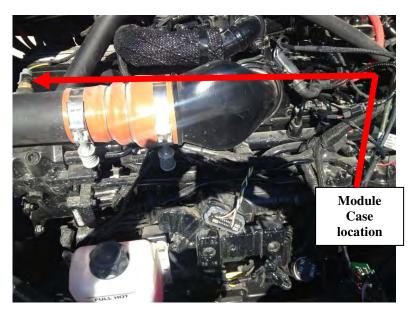
**4)** On the Ag Diesel Solutions harness, the male injector connector located closest to the module case will connect to the female injector connector wiring located closest to the flywheel-side of the engine.
