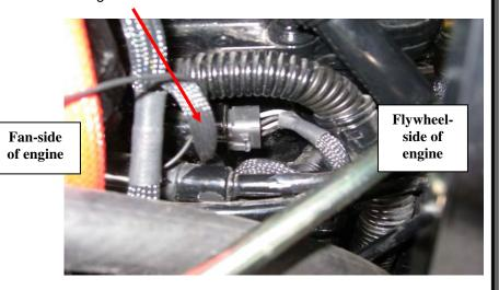
**6)** Continue to the next 2 sets of injector plugs. Repeat Steps 4 and 5 to connect each pair of injector plugs. Note: The new harness will connect in series between the stock injector plugs and stock wiring plugs. All plugs on the new harness will be connected.
