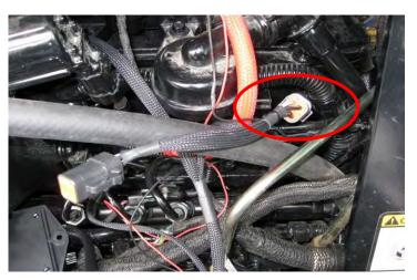
**5)** On the Ag Diesel Solutions harness, the male injector connector located closest to the module case will connect to the female injector connector located closest to the flywheel-side of the engine.
