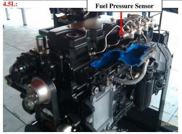
2) Locate fuel pressure sensor as shown above. It can be located at either end of the common rail or protuding outward in the middle
