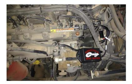
6) Mount the module in a secure location away from any extreme heat or moving parts as shown above. Strap the module to a factory wiring harness and tie any excess harness down.
