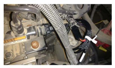
4) Insert the Female Connector from the ADS module harness into Fuel Pressure Sensor.
