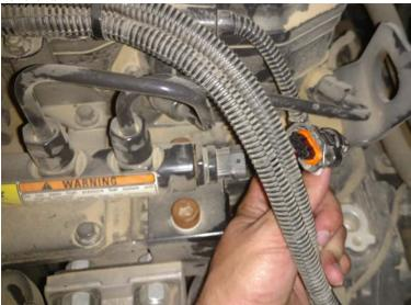
**3**) Disconnect the fuel pressure sensor connector. This is a 3-Pin connector.
