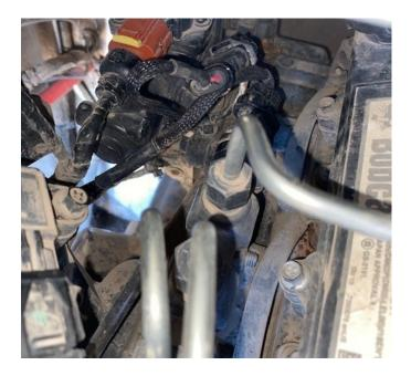
**5)** Mount module in a secure location away from any extreme heat or moving parts. Zip tie module and any loose wires down.
