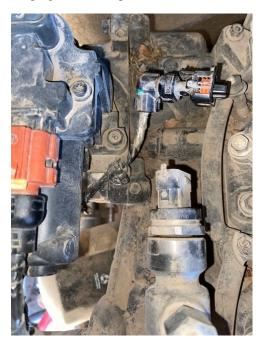
**4)** Plug the 3-pin male connector from module into the stock fuel pressure sensor. Connect the stock 3-pin male fuel pressure connector to the female 3-pin connector on the ADS module harness.
