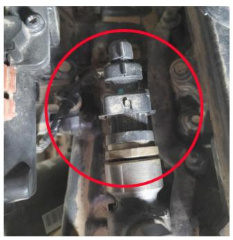
3) Unplug the stock 3-pin male connector to the fuel pressure sensor.
