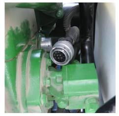
3) Unplug the factory injector connector and plug in male Injector connector from the Ag Diesel Solutions module into the head.4) Plug the stock connector to the female injector connector from the Ag Diesel Solutions module.
