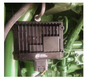
**10)** Mount the module with the connector on the bottom side, as to reduce the chance of moisture from getting into the module harness. Keep away from excessive heat and moving parts.
