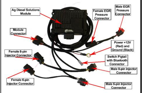
1) Locate the 2 fuel injector connectors as shown in the picture below.
