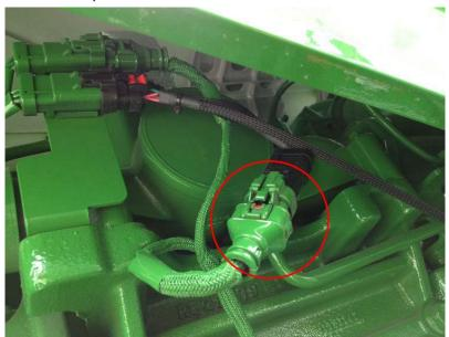
6) Plug the female Ag Diesel Solutions exhaust pressure connector into the stock exhaust pressure connector. Note: Slide red locking tab
