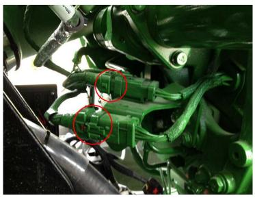
3) Unplug both injector connectors and plug the stock injector connectors into the male connectors on the Ag Diesel module harness. Plug the female Ag Diesel Module connectors into the stock male connectors. Note: There are locking tabs on each connector. Slide the locking tab away from connector to unlock and toward the connector to lock.
