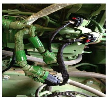
4) From inside the cab facing forward, locate the EGR pressure connector on the driver's side of engine, it is located toward the top of the engine. There are 2 connectors in this location, the EGR pressure connector is the bottom connector.
