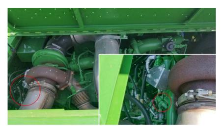
To locate the EGR pressure connector, lift the second access panel closest to the grain bin. The EGR pressure connector can be found under the cutout in the sheet metal panel as shown below.
