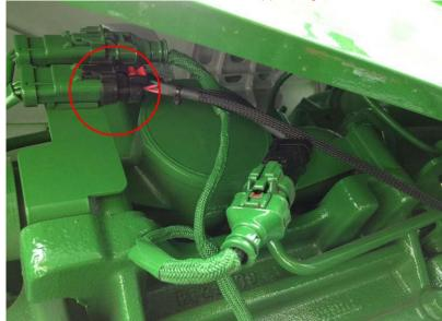
7) Locate the starter. onnect the red wire with ring terminal to 12 volt source on starter. Connect the black wire w/ring terminal to ground on starter. Note: When routing wiring, secure and zip tie the wiring in place keeping away from exhaust or any rotating parts.
