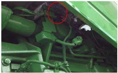
**5)** Unplug the stock EGR pressure connector. Plug the stock male EGR pressure connector into the female Ag Diesel Module EGR pressure connector.
