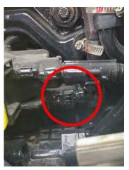
**3)** Connect the 3-Pin male fuel pressure connector on the Ag Diesel Solutions Module to the stock 3-Pin female connector on the engine. Then connect the stock 3-Pin male connector on the engine harness to the 3-pin female connector on the Ag Diesel Solutions module Harness.
