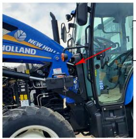
Fuel Pressure sensor location. **2)** Locate the fuel pressure sensor. It can be located at either end of the common rail or protruding outward in the middle of the rail. This is a 3-Pin connector.
