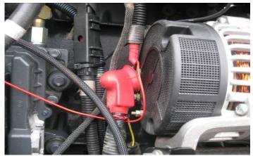
**9)** Plug the harness into the module. Mount the module with supplied zip ties away from any excessive heat or moving parts. Note: Zip tie the module to the factory wire harness. Mounting the module with the switch connector down will help prevent moisture from collecting into the module connector.
