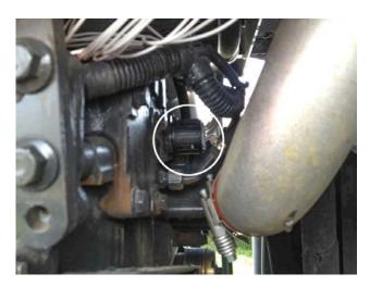
3) Plug the female connector from the Ag Diesel Solutions module into the stock location on the engine head. Align the inside section of the connector to the stock plug and then rotate the outer shell clockwise to tighten. Note: The outer shell spins free of the inside connector. Align the inside section and then rotate the outer shell until the connector snaps.
