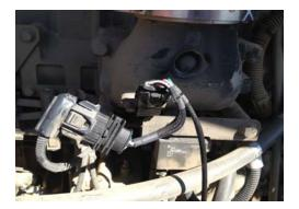
7) Connect the Black wire with Ring Terminal to a good chassis ground
