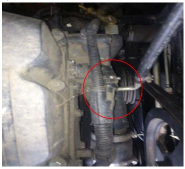
**3)** Plug the female connector from the module harness into the male stock connector. Plug the male connector from the module harness into the side of the engine head. Rotate housing to lock connector in place.
