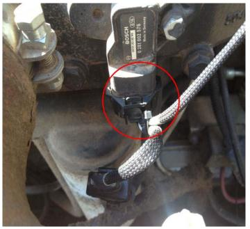
7) Connect the Black wire ring terminal to a good chassis ground. Connect the Red wire ring terminal to a +12V constant source (i.e. alternator).
