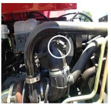
**8)** Connect the black wire with ring terminal to a good chassis ground. Connect the red wire to the alternator 12v constant power.
