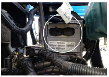
**4)** Plug the male connector from the module into the 16 pin ECM port as shown below.
