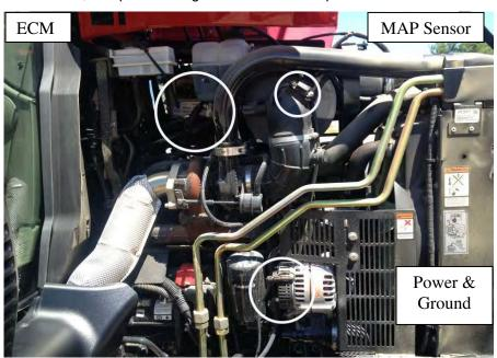
**3)** Press the locking lever on the ECM connector and unplug both the left and right ECM connectors as shown.
