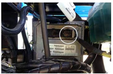
**5)** Plug the stock ECM connector that was removed in Step 3. Plug the stock connector to the female connector from the module harness.
