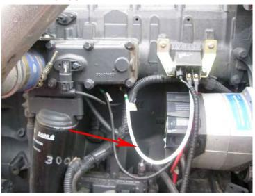
**8)** Connect Red wire with ring terminal to a 12V constant source (i.e. alternator).
