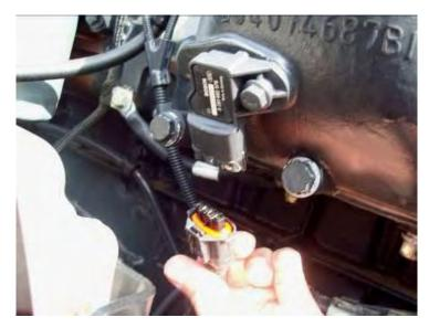
**6)** Plug the stock male MAP connector into the female connector from the module.
