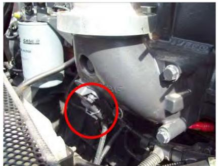
**5)** Unplug MAP sensor and plug the male connector from the Ag Diesel Solutions module into the stock MAP sensor.
