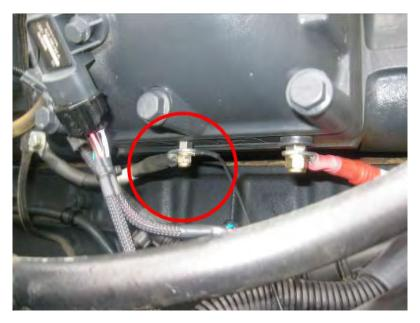
Note: Do **NOT** Connect to white wire coming from relay to bottom of intake manifold
