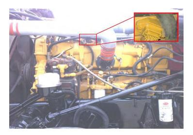
2) Plug the male connector from the Ag Diesel Solutions module into the stock female connector on the engine. Plug the stock injector harness, that was removed in Step 1, into the female connector from the Ag Diesel Solutions module. Note: There are 2 keys located on one side of the male and female plugs. Line up the keys when connecting.
