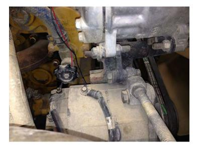
8) Plug the Harness into the module. Mount the module with supplied zip ties away from any excessive heat or moving parts. Note: Zip tie the module to the factory wire harness. Mounting the module with the switch connector down will help prevent moisture from collecting into the module connector
