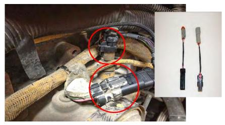
**7)** Route the power and ground wires to the alternator. Connect the red wire to +12 volts constant and the black wire to Ground.
