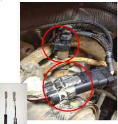
**4)** Unplug the Stock MAP Sensor and then Proceed to Step 5. Note: If your MAP sensor is the same style as what is shown in the below picture, the MAP Sensor jumpers supplies with your module will not be used.
