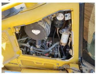
2) Locate fuel pressure sensor as shown below. It can be found at the end of the fuel rail closest to the firewall.
