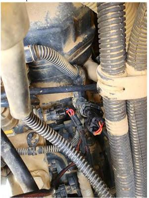
**5**) Connect the Stock Cummins connector to the Male Fuel Pressure Connector on the module harness.
