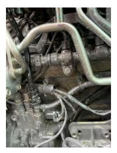
2) Locate the fuel pressure sensor as shown in the picture above. The sensor is located at the end of the common fuel rail.
