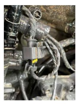
**4)** Plug the 3-pin male connector from module into the stock fuel pressure sensor. Connect the stock 3-pin male fuel pressure connector to the female 3-pin connector on the ADS module harness.
