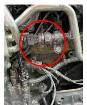
3) Unplug the stock 3-pin male connector to the fuel pressure sensor.
