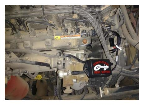
5) Mount the module in a secure location away from any extreme heat or moving parts as shown above. Strap the module to a factory wiring harness or tubing and tie any excess harness down.
