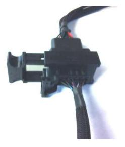
4) Connect the stock female pump connector to the male pump connector on the Ag Diesel Solutions module harness.
