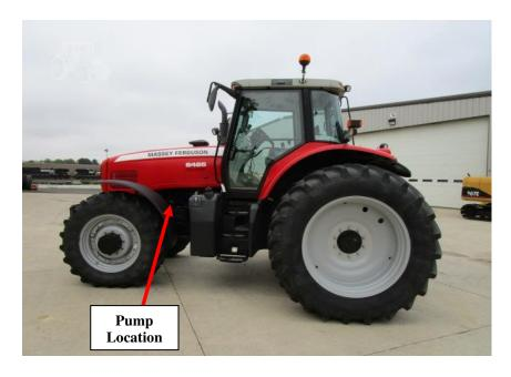
1) From the tractor cab looking forward, locate the pump on the left side of the engine. You will see the injector lines coming out of it.
