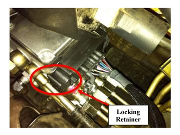
2) Locate the big connector on the pump. Slide the locking retainer out and remove the wiring harness.
