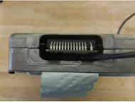
The proper orientation of the chip is with the circuit board of the chip and the switch cable on the larger side of the J3 port opening.
