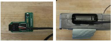
The proper orientation of the chip is with the circuit board of the chip and the switch cable on the larger side of the J3 port opening.
