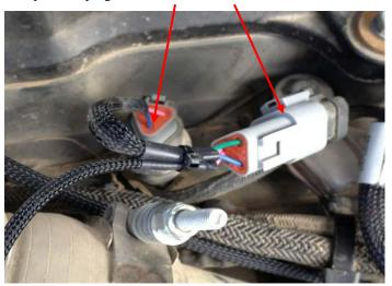
Note: If your MAP sensor has the gender connector shown in picture B then you will not need to use the jumpers. If your MAP sensor has the gender connector shown in picture A then you will need to use the jumpers provided (picture C)
