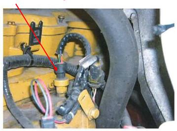
5) Disconnect the MAP Sensor and plug the Male plug from the module into the stock MAP/Boost Sensor.
