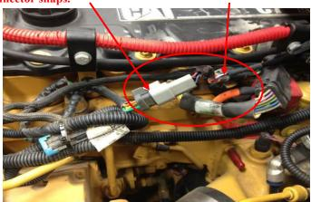
**4)** Locate the Map sensor on the Intake Manifold on the driver's side of the engine. Refer to the diagram on Page 2 for approximate location.
