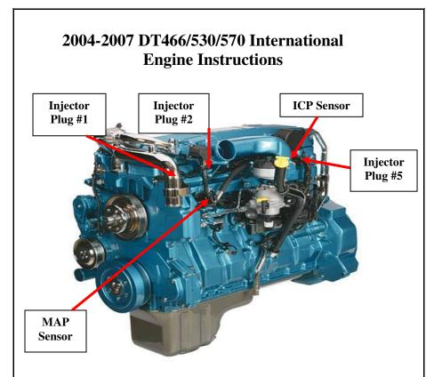
1) Locate the MAP Sensor on the driver's side of the engine. Refer to the picture above for location.
