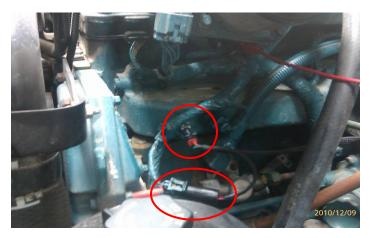
3) In order to locate the ICP Sensor, find each of the 6 Injector Plugs on the driver's side of the engine head. Starting with Injector Plug #1, as labeled in the picture on page 3, count each one until you reach the #5 Injector plug. The ICP Sensor is located next to the #5 Injector plug.
