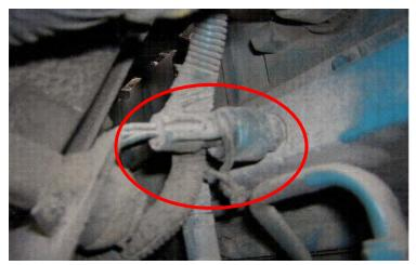
2) Unplug the stock connector from the MAP Sensor. Plug the stock male connector into the female connector on the module harness. Plug the male connector from the module harness into the stock MAP Sensor.
