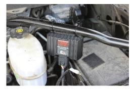
7) Route Switch through firewall and plug into the module harness as shown.
