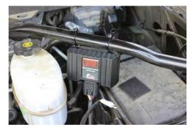
9) Connect module switch harness. Based on preference, the module switch can be secured in the engine compartment near the module or it can be routed into the cab. If mounting in the cab, route the Switch through the firewall and connect to the module harness.
