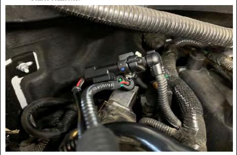
5) Disconnect the stock male MAP Sensor connector from the MAP Sensor.
