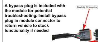
Make sure to push completely together until connector snaps when using bypass plug.
