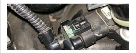
**6)** Utilize the portion of the Ag Diesel Solutions harness labeled MAP. Connect the male connector to the MAP Sensor. Then connect the female connector to the stock male MAP Sensor connector.
