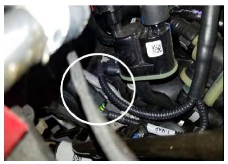
7) Remove the bypass plug from the Ag Diesel Solutions harness, and plug the harness into the module.
