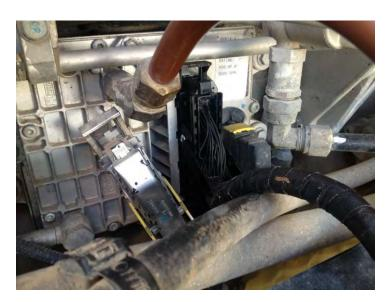
**4)** Connect the Ag Diesel Solutions female harness into the stock female plug located on the engine harness. Squeeze the connector together and then press the locking lever to latch the
