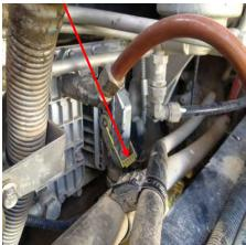
**3)** Connect the male connector from the Ag Diesel Solution module harness into the ECM.
