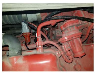
**5)** Continue to the next injector connector. Repeat Step 4 to connect each pair of injector connectors. Note: The new harness will connect in series between the stock injector plugs and stock wiring plugs. All plugs on the new harness will be connected.
