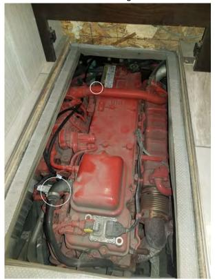
**2)** Unplug both sets of stock injector connectors. Press the release tab on the connector and gently pull the connector apart.
