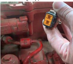
**3)** Route the Module Harness as shown in the picture below. The Module Case will be located closer to the Fan side of the engine.
