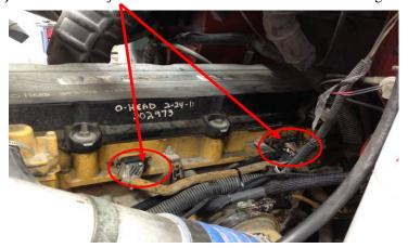
2) Unplug the stock injector connector located closest to the firewall.
