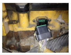
3) Plug the male connector from the module into the stock connector on the engine head. Plug the stock male connector into the female module harness connector
