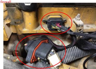
**4)** Follow Steps 2 and 3 for the second injector connector located closest to the engine fan.
