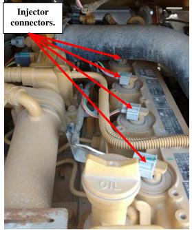
2) Disconnect all four of the stock injector connectors. Press and hold the release tab on the connectors and gently pull the connectors apart.
