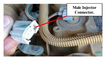
3) On the module harness, the male connectors will connect to each individual injector. Injector connector 4 will connect to the injector closest to the flywheel. They will then connect in order with connector 1 ending on the injector closest to the fan/serpentine belt.
