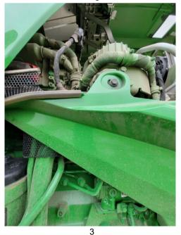
**2)** Locate the injector connector near the top of the engine, behind the boost tube.
