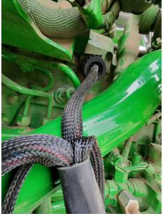
**4)** Plug the factory male connector into female module injector connector.
