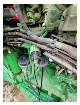
Locate the MAP sensor on the top center of the engine.
