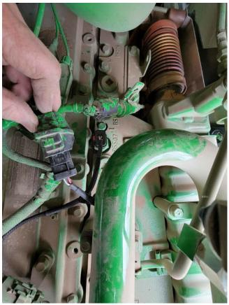
**Note:** Make sure to push completely together until the connector snaps.
