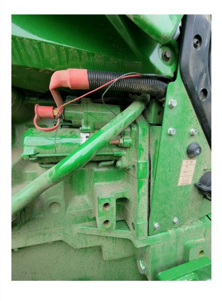
**10)** Plug the harness into the module. Mount the module with supplied zip ties away from any excessive heat or moving parts. Note: Zip tie the module to the factor wire harness. Mounting the module with the switch connector down will help prevent moisture from collecting into the module connector.
