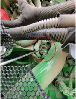
**3)** Unplug the injector connector by twisting the cam lock counter clockwise. Install module male connector into factory injector connector.
