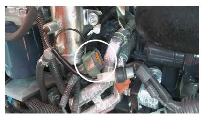
**7)** Plug the male EGR valve connector from the Ag Diesel Solutions module harness into the stock female EGR valve. Plug the male EGR valve connector from the stock harness into the female Ag Diesel Solutions EGR valve connector.
