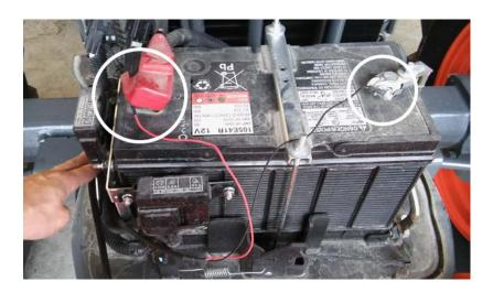
**9)** Plug the harness into the module. Mount the module with supplied zip ties away from any excessive heat or moving parts.
