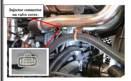
**4)** On the Ag Diesel Solutions module harness, the gray 10 pin female injector connector will now plug into the factory male injector connector that was unplugged from the valve cover in Step 2.
