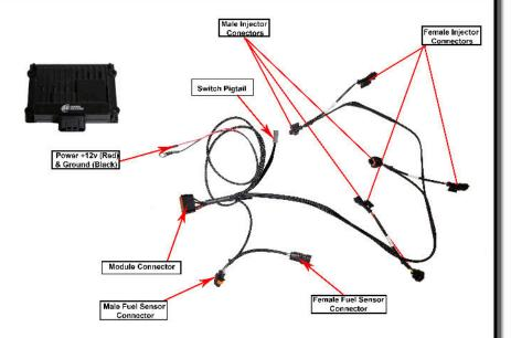
**1)** On the drivers side, under the hood, locate the fuel sensor connector and the 3 injector connectors.
