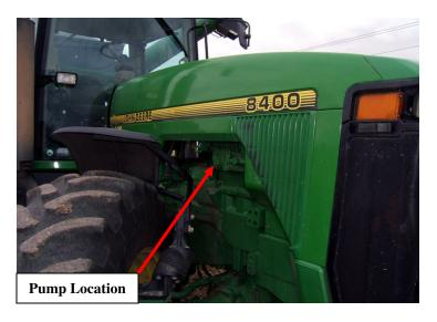
1) Locate Bosch P-pump on left side of tractor beside the front tire, if you're facing the front of the tractor.
