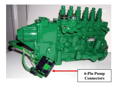
2) Locate the 6-Pin fuel pump connector coming off of the back of the fuel pump as shown in the picture above.
