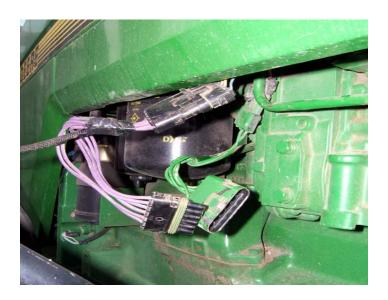
**4)** Insert the factory Male fuel pump connector into the Female connector on the ADS module harness.
