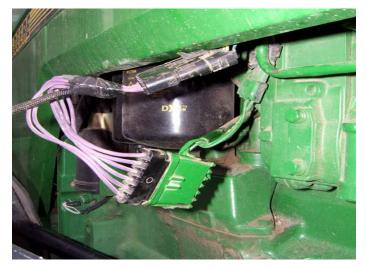
**5**) Insert the Male connector from the ADS module harness into the factory Female fuel pump connector.
