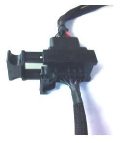
4) Connect the stock Female pump connector to the Male pump connector on the ADS module harness.
