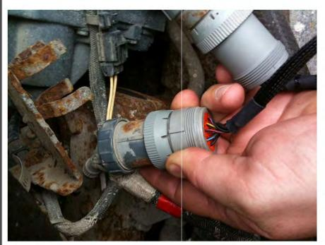
4) Plug Male Module Connector into the stock Female Mack harness.
