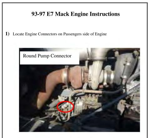
2) Unplug round engine connector as seen in picture
