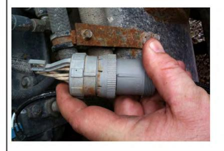
5) Route Switch through the firewall and plug into module as shown
