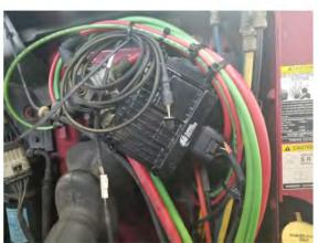
**11)** Route the power and ground wires to the alternator located on the passenger's side of the engine. Connect the red wire to +12 volts and the black wire to Ground.
