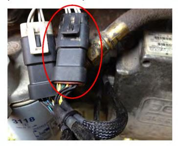
**9)** Connect the module black injector connector into the stock ECM. It will plug into the top ECM connector.
