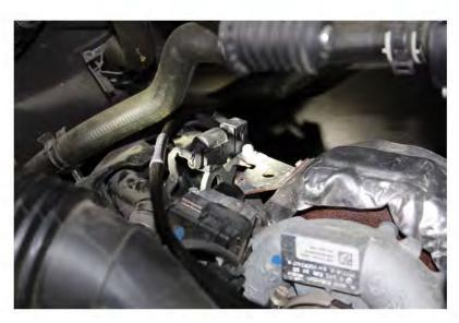
**5)** Plug male stock fuel pressure sensor connector into female Truck Edition fuel pressure connector.
