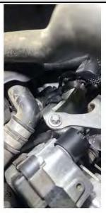
**4)** Plug male Truck Edition fuel pressure connector into the factory fuel pressure sensor. Apply even pressure until connector clicks into place.
