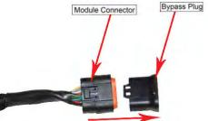
Mount the module in a safe location using the zip ties to secure the wires and module away from extreme heat and moving parts.
