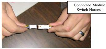
7) Remove the bypass plug from the Ag Diesel Solutions harness, and plug the harness into the module.
