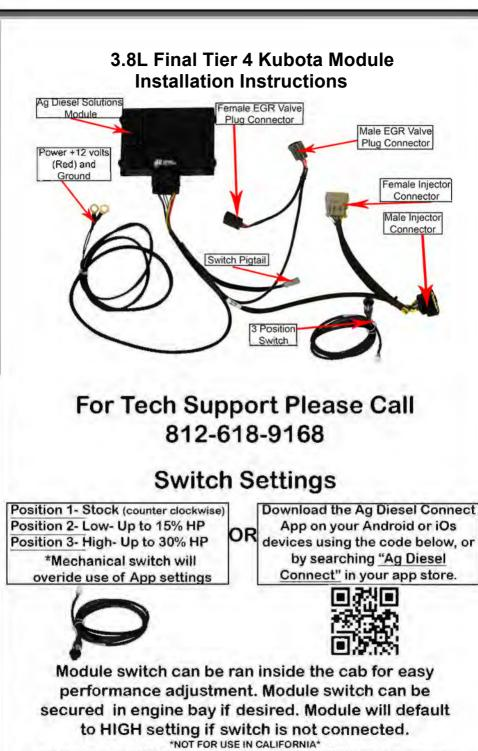
\*MODULE DOES NOT BYPASS, DELETE, OR DEFEAT ANY EMISISON CONTROL SYSTEMS\* \*If installation assistnace is needed, Ag Diesel Solutions is not responsible for any cost associated with third party installation. **1)** Locate the stock injector connector on top of the valve cover. This is accessible from the right hand side of the engine. This is a ten pin connector that will be enclosed in a protective rubber weather seal.
