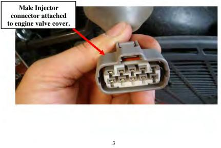
**3)** On the Ag Diesel Solutions module harness, the white 10 pin male injector connector will connect to the female injector connector fixed on the valve cover as seen in Step 1. The module harness can be routed along existing wire loom.
