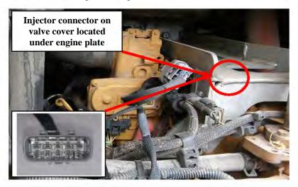
**4**) Plug the factory male injector connector, that was unplugged from the valve cover in Step 2, into the module harness.
